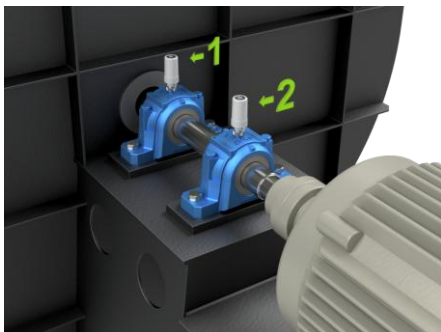
Sensor placement for overhung component
