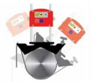
Three readings are required in order to determine the machine's position. The tripoint method provides a quick and easy way to register the readings. The result is instantly displayed on the screen with all relevant information.
