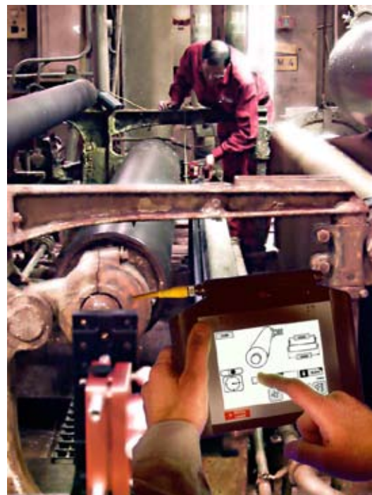
Roll parallel measurements being performed with the Fixturlaser Roll 200 by plant maintenance personnel.
